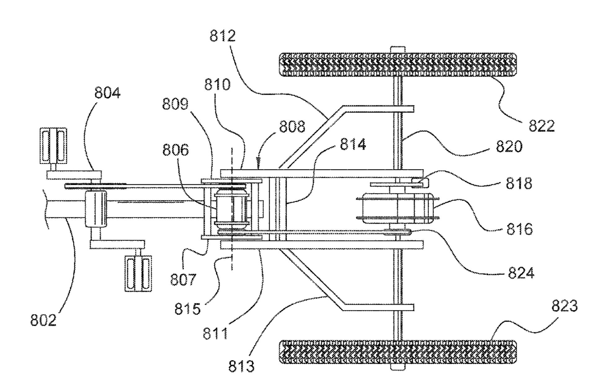
belt. The transmission has an output that is coupled to a rear wheel assembly. In some embodiments the rear wheel assembly can be mounted in a swingarm that pivots about a transverse axis defined by the output of the transmission. In some embodiments the rear wheel assembly can include an electric motor to drive a rear wheel.
