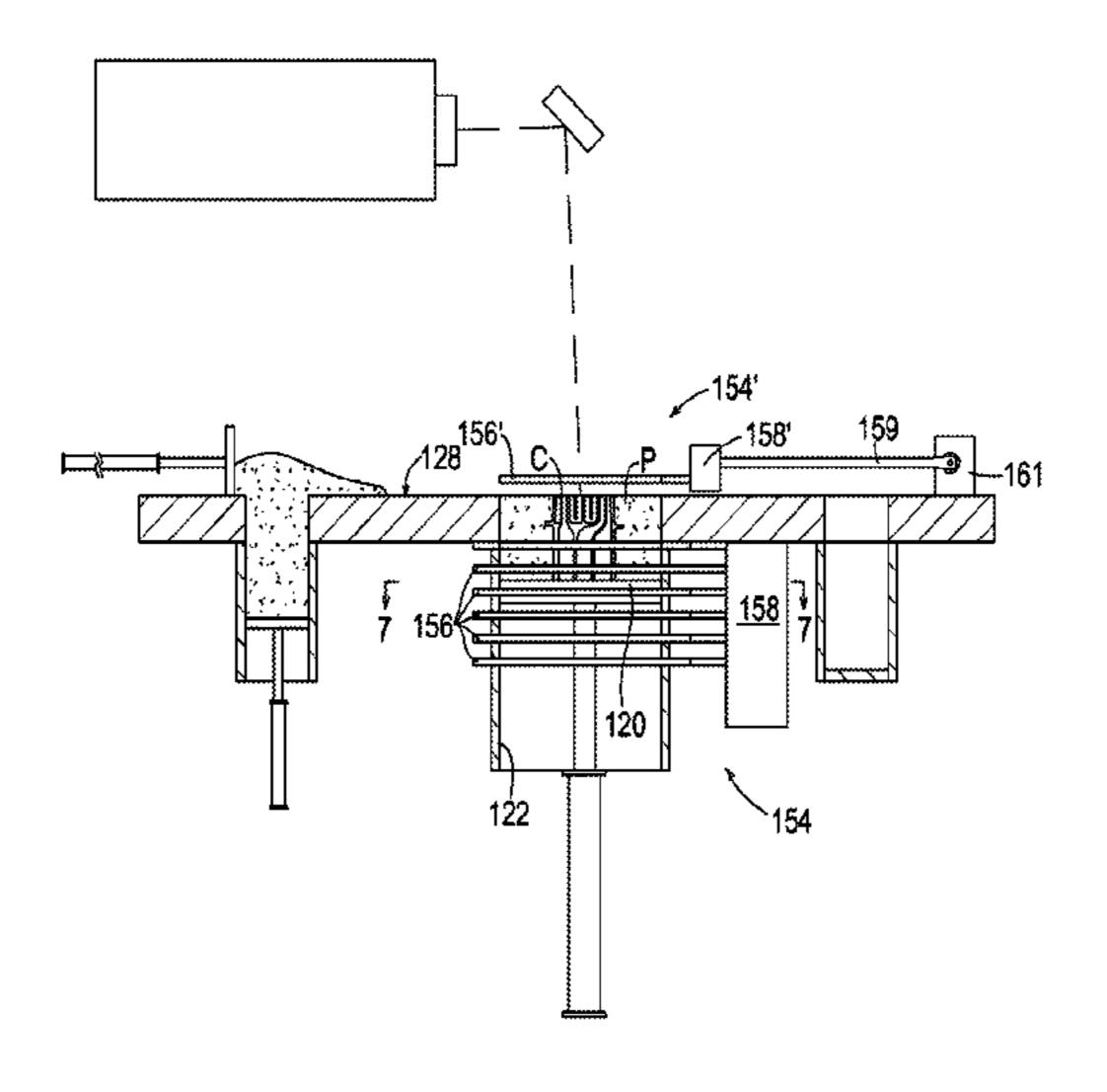
heat control apparatus separate from the directed energy source to maintain a predetermined temperature profile of the component, such that the resulting component has a directionally-solidified or single-crystal microstructure.
