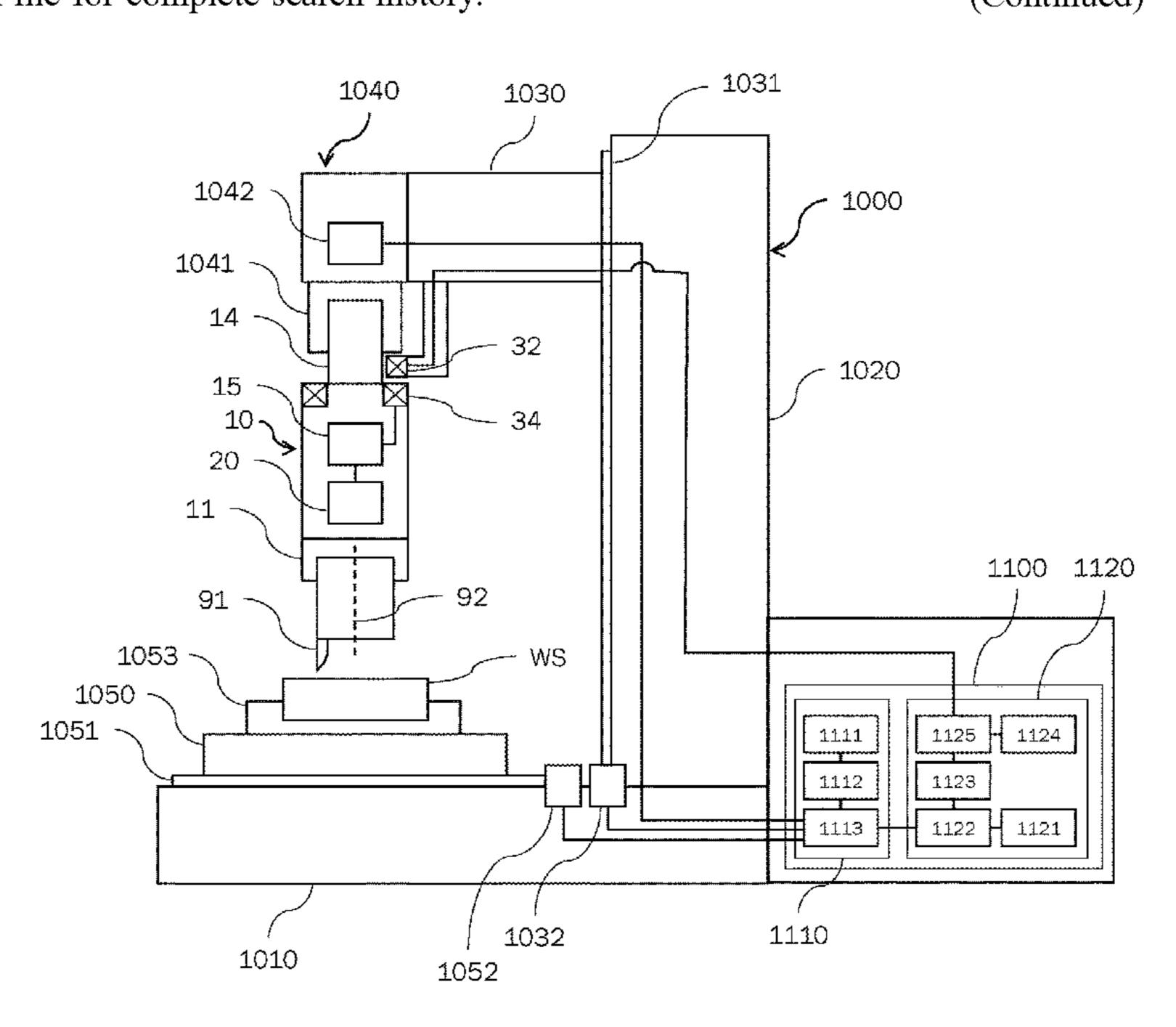
milling cutter on the basis of a control signal to an actuator which is integrated in the tool head and is configured to drive a vibration of the milling cutter on the basis of the control signal, wherein the control signal contains high-frequency carrier signal and a useful signal which modulates the carrier signal and which is generated on the basis of data indicating the predetermined pattern.
