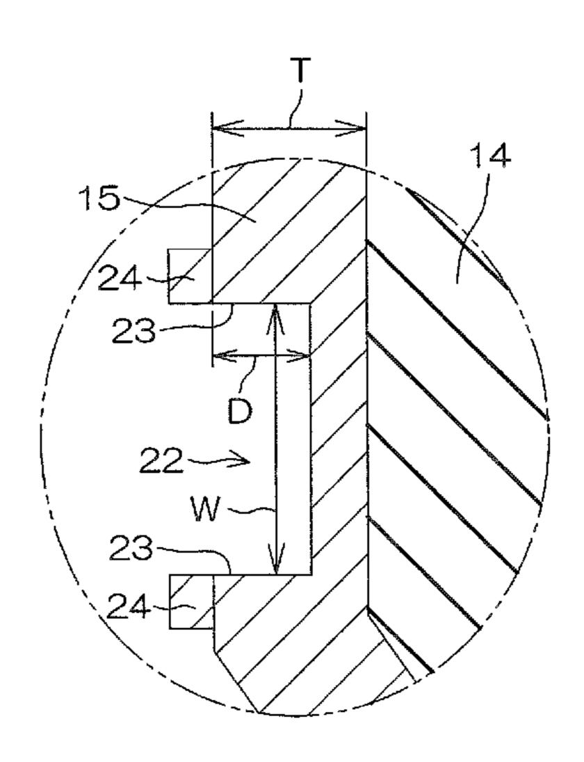
surface portion in the mold with the gasket being laminated with a lamination film; and demolding the gasket from the mold, and then forming a groove only in the lamination film circumferentially of the circumferential surface portion of the gasket.
