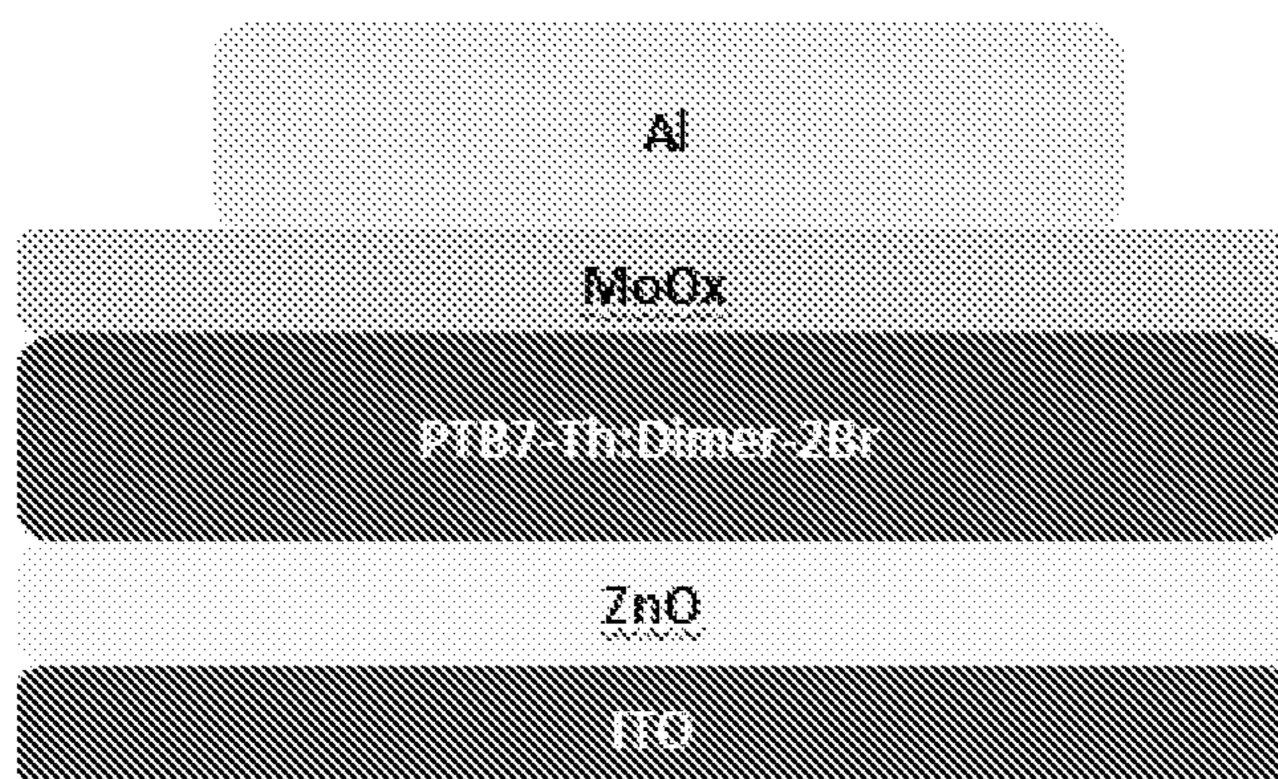
Device structure (inverted)
