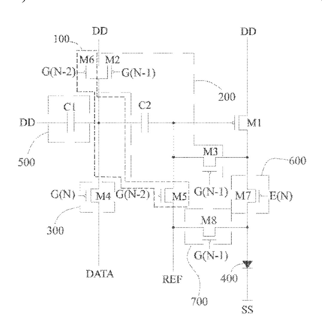
the driving sub-circuit, a third terminal, and a fourth terminal, and a control terminal. The data writing sub-circuit includes a first terminal and a second terminal. The data voltage storage sub-circuit includes a first terminal electrically coupled to the third terminal of the compensation sub-circuit and the second terminal of the data writing sub-circuit; and a second terminal.
