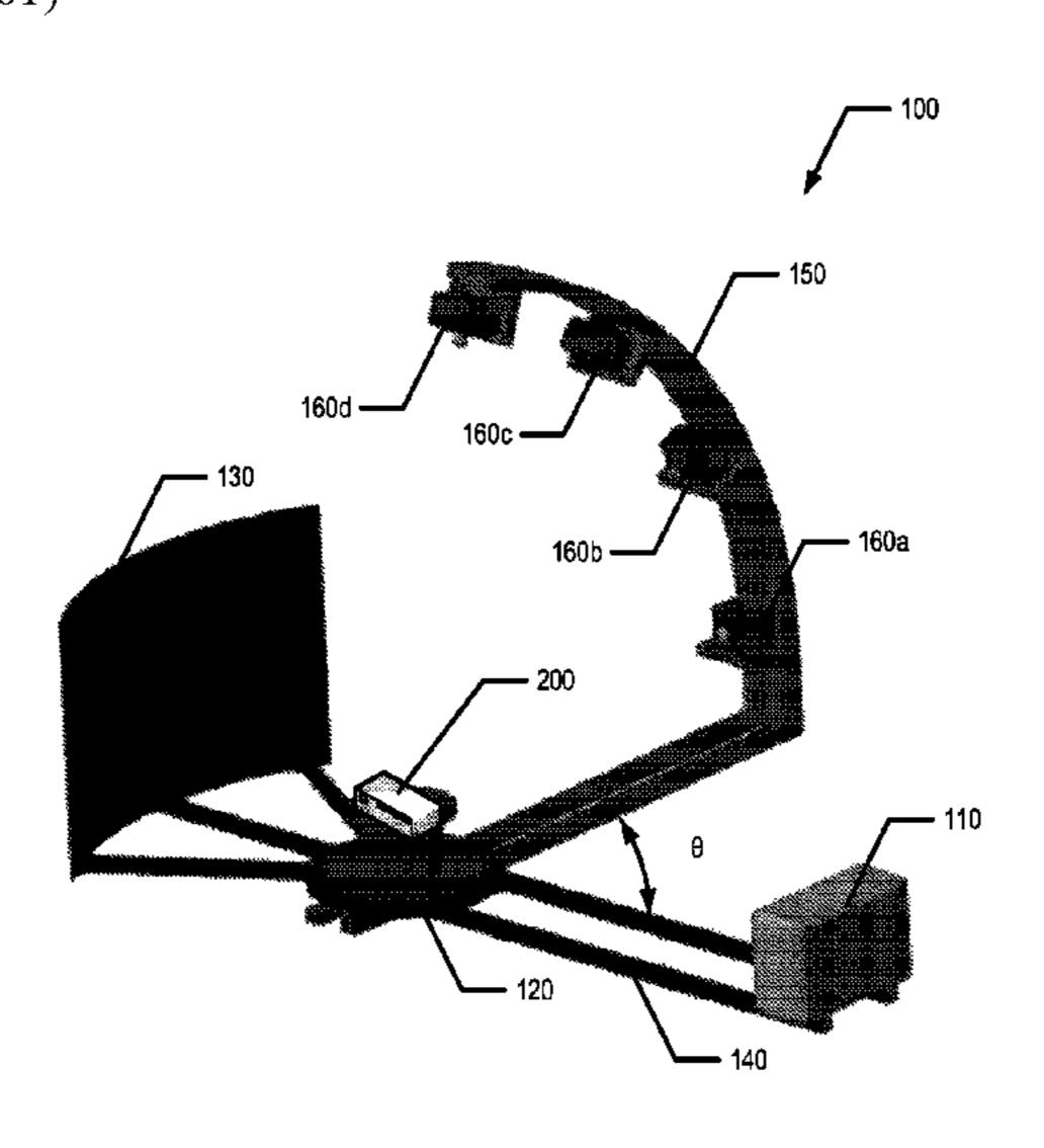
object with the light source; and with each spectrograph, capturing a reflectance spectra associated with the object. The turntable is rotated such that an azimuthal angle between the object and the light source is changed. The capturing and rotating steps are repeated for a predetermined set of azimuthal angles.
