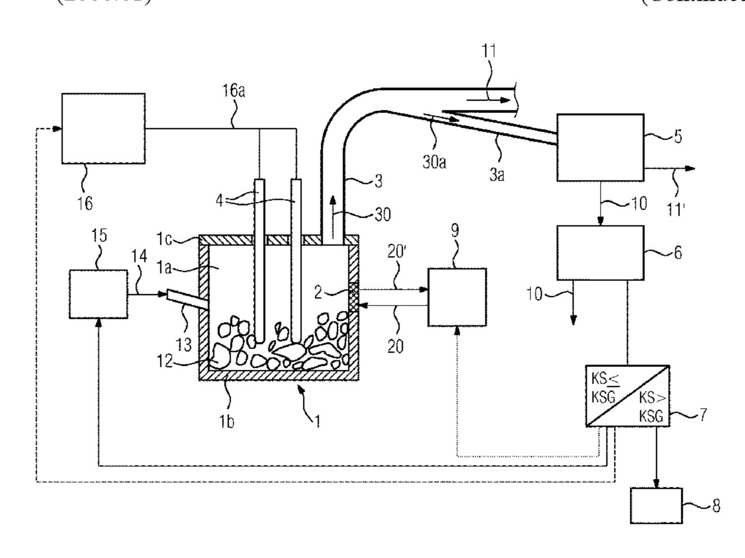
mining a stream of condensate obtained; comparing the stream of condensate obtained with a condensate-stream limit value; and indicating a leakage if the stream of condensate exceeds the condensate-stream limit value. Also a device for carrying out the method and a furnace with such a device are disclosed.
