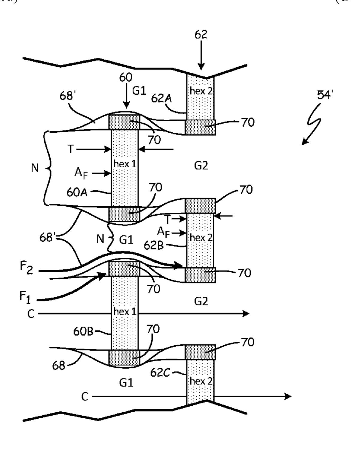
exchanger. Each neck region has a neck area that is less than a frontal area of the heat exchanger with which it is aligned.
