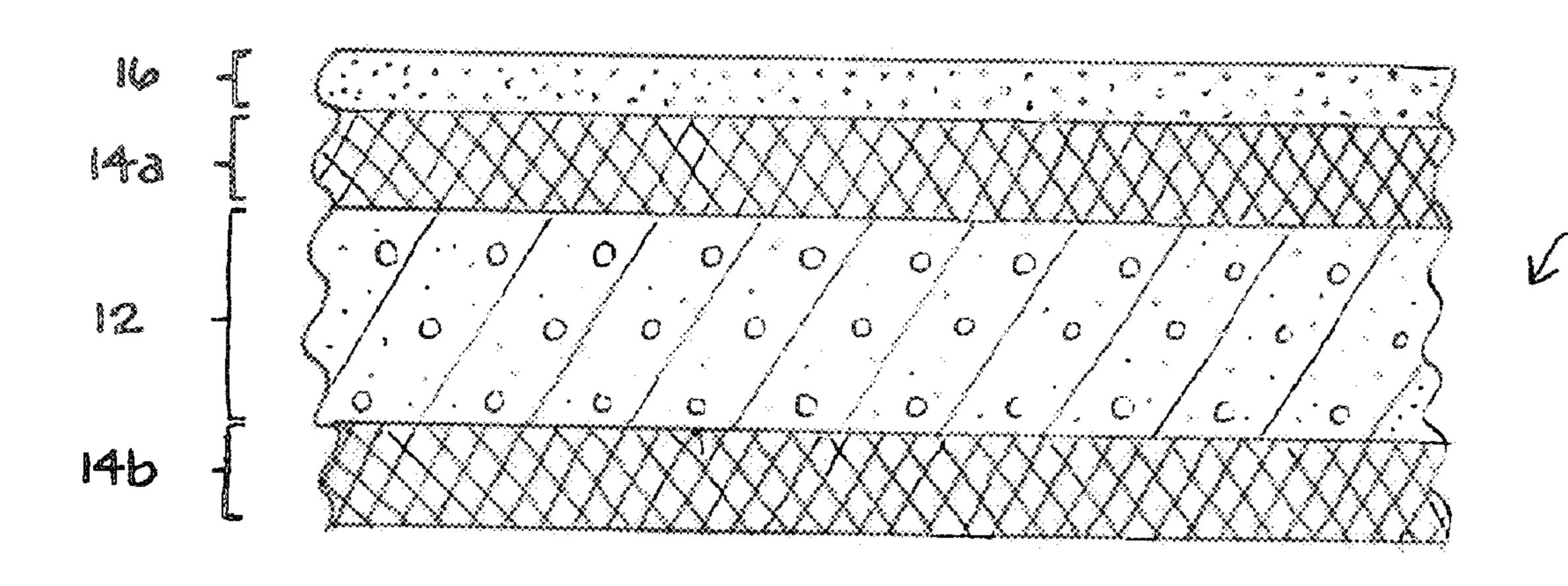
manufacturing exterior sheathing cementitious panels with a highly efficient integrated air/water barrier membrane are provided as well.
