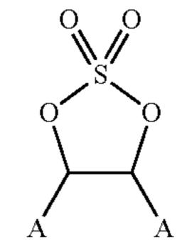
wherein each A is independently a hydrogen or an optionally fluorinated vinyl, allyl, acetylenic, propargyl, or  $C_1$ - $C_3$  alkyl group. The electrolyte compositions are useful in electrochemical cells, such as lithium ion batteries.
