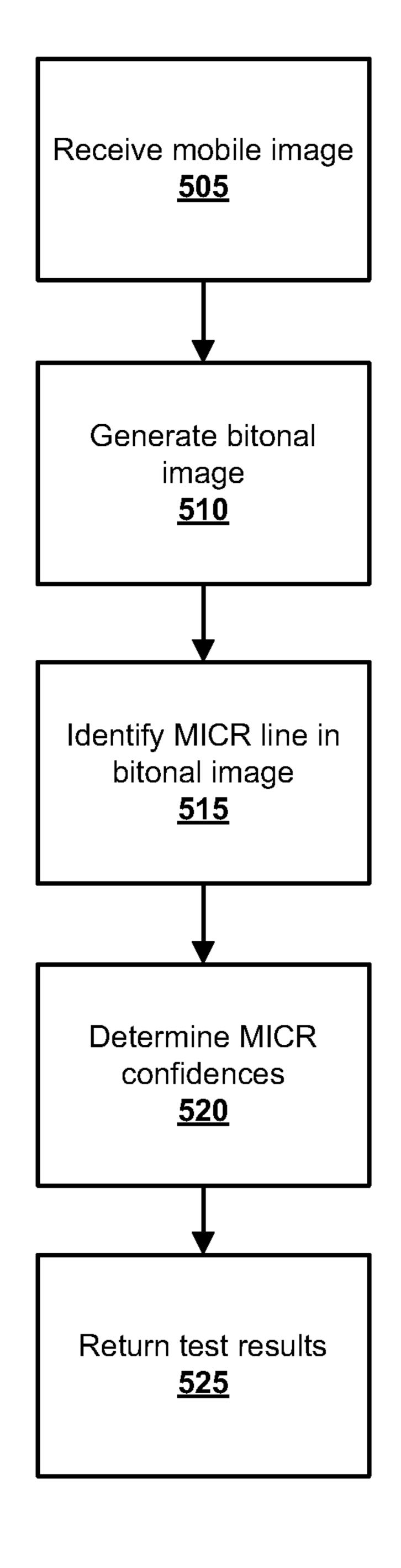
FIG. 5 MICR-line Test
