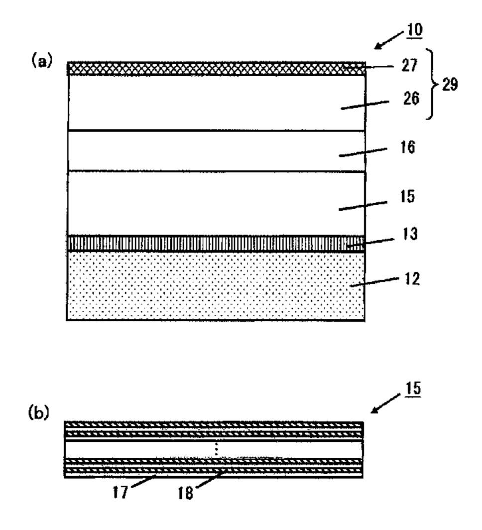
lower surface of the buffer layer, and an iron concentration of the upper surface of the buffer layer is lower than an iron concentration of the lower surface of the buffer layer. As a result, the substrate for semiconductor device can reduce a leak current in a lateral direction at the time of a high-temperature operation while suppressing a leak current in a longitudinal direction.
