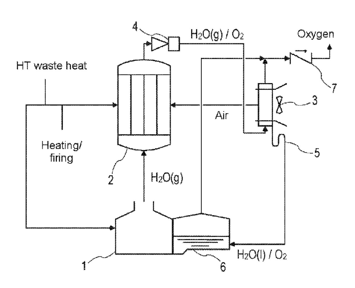
according to the invention water in various aggregate states is conducted in a circuit and the configuration of the equipment is designed such that the desired high oxygen pressure is produced in a separate area from the membrane module and the oxygen produced is prevented from mixing with the freshly produced water vapour.
