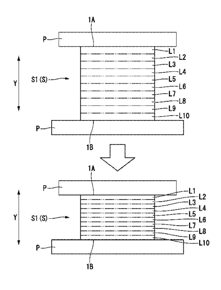
thickness ratio in the vertical direction (Y) among the plurality of layer parts (L1 to L10).
