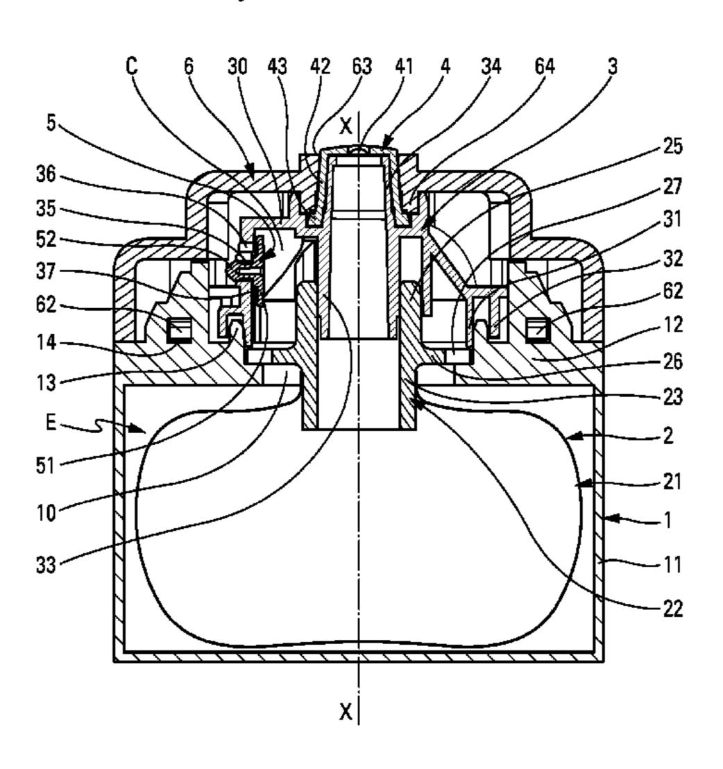
shell (1) and on the flexible inner pouch (21), the hood (6) including a window (63) in which the dispenser valve (4) is positioned.
