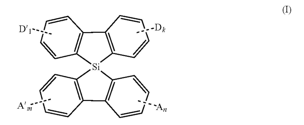
as compounds capable of emitting delayed fluorescence, and uses of the compounds in organic light-emitting diodes.
