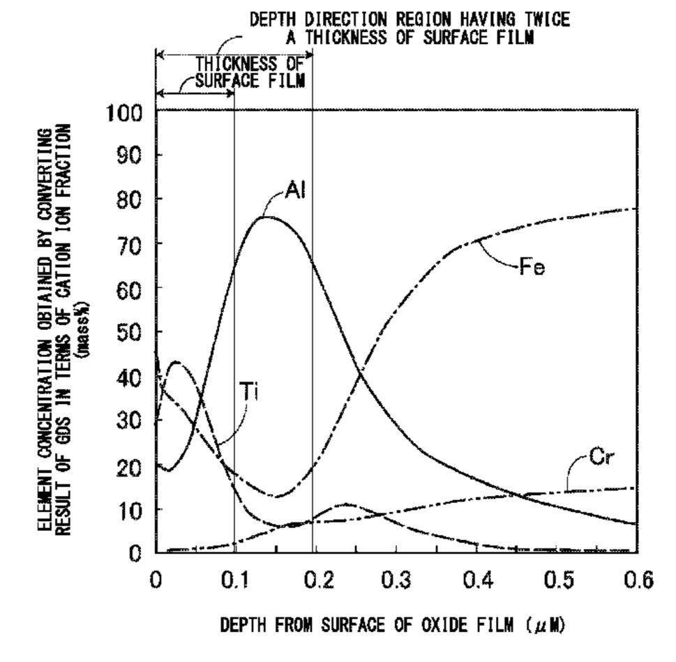
ion fraction excepting O in an depth direction region having twice a thickness of an oxide film having less than  $0.1 \mu m$ .
