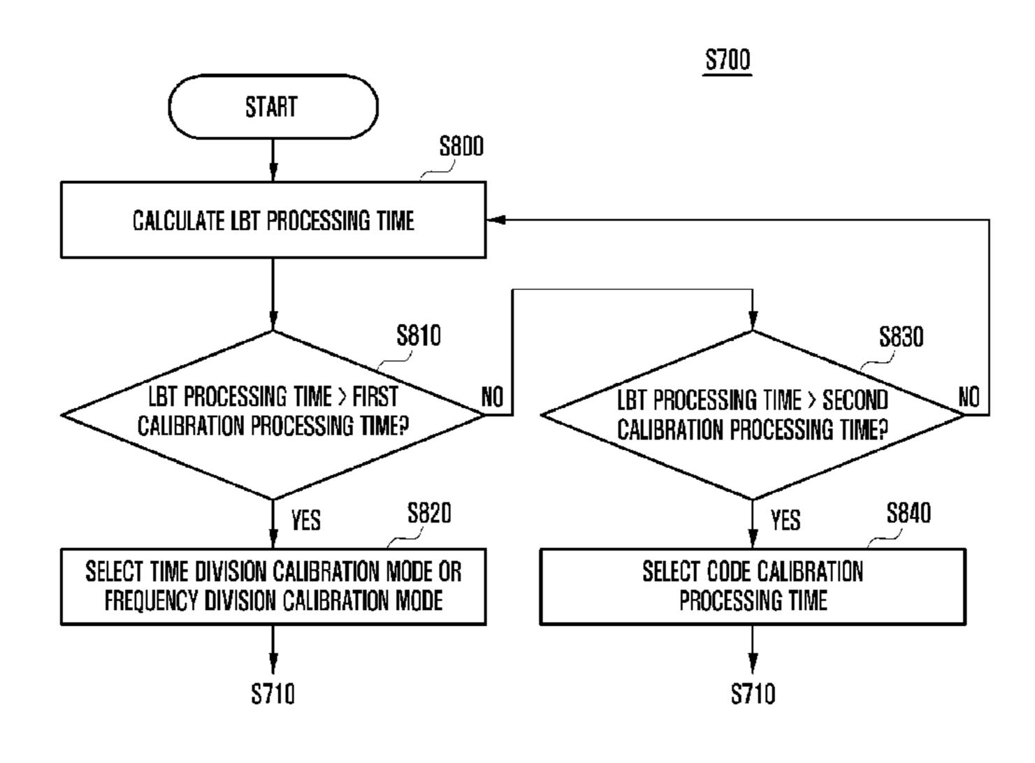
inter-antenna phase on the basis of the LBT processing time; and calibrating the inter-antenna phase according to the selected calibration mode.
