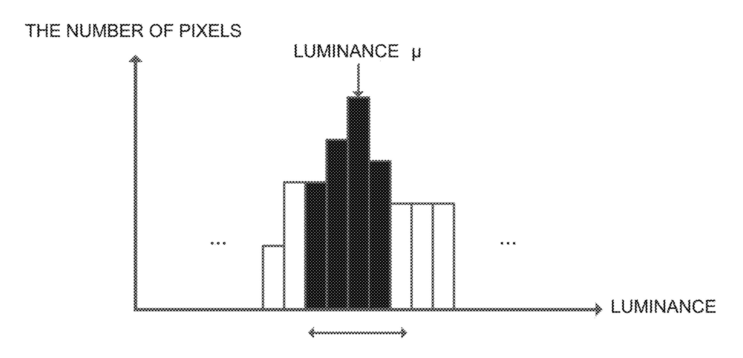
SEQUENTIALLY ADDING ZONE OF LUMINANCE, RESPECTIVELY, BEFORE AND AFTER THE ZONE OF LUMINANCE  $\mu$  FOR HISTOGRAM TO DETERMINE THE MINIMUM ZONE (BLACK REGION) WHERE THE SUM OF THE NUMBER OF PIXELS CONTAINED IN THE CONNECTED ZONES COMES BEYOND M (THE NUMBER OF EXTRACTED PIXELS)
