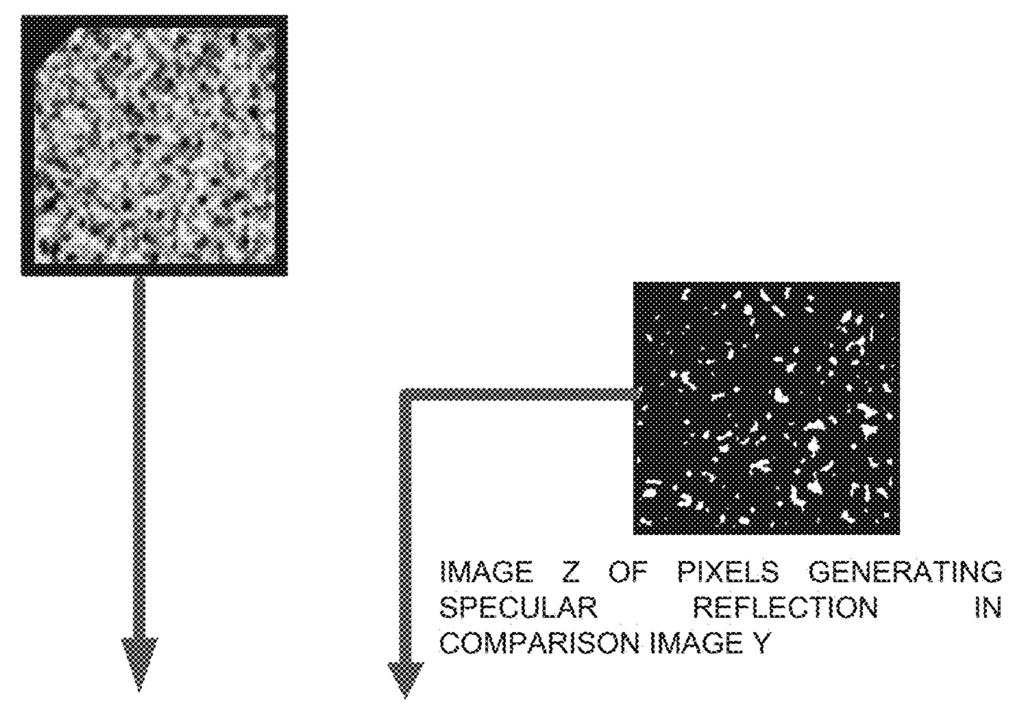
EXTRACTING PIXELS AT POSITIONS CORRESPONDING TO PIXELS ESTIMATED TO BE GENERATING SPECULAR REFLECTION IN COMPARISON IMAGE Z FROM REGISTERED IMAGE X
