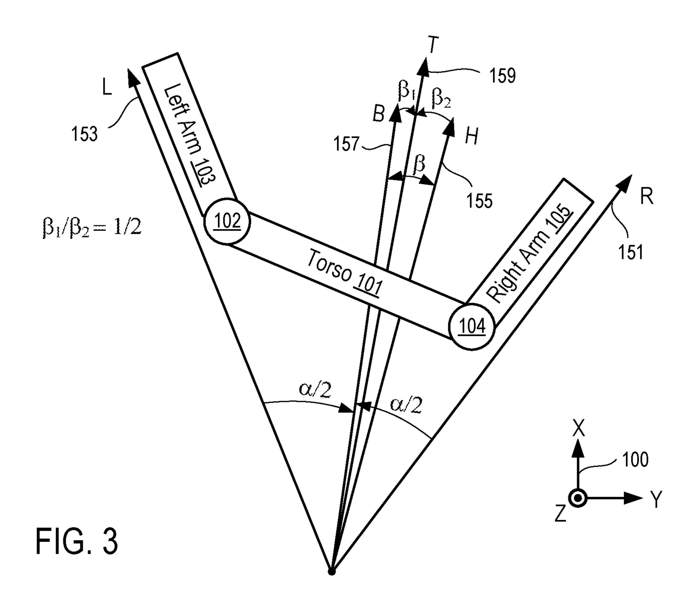
Receive motion data from two arm modules identifying orientations of the upper arms of a user 201
