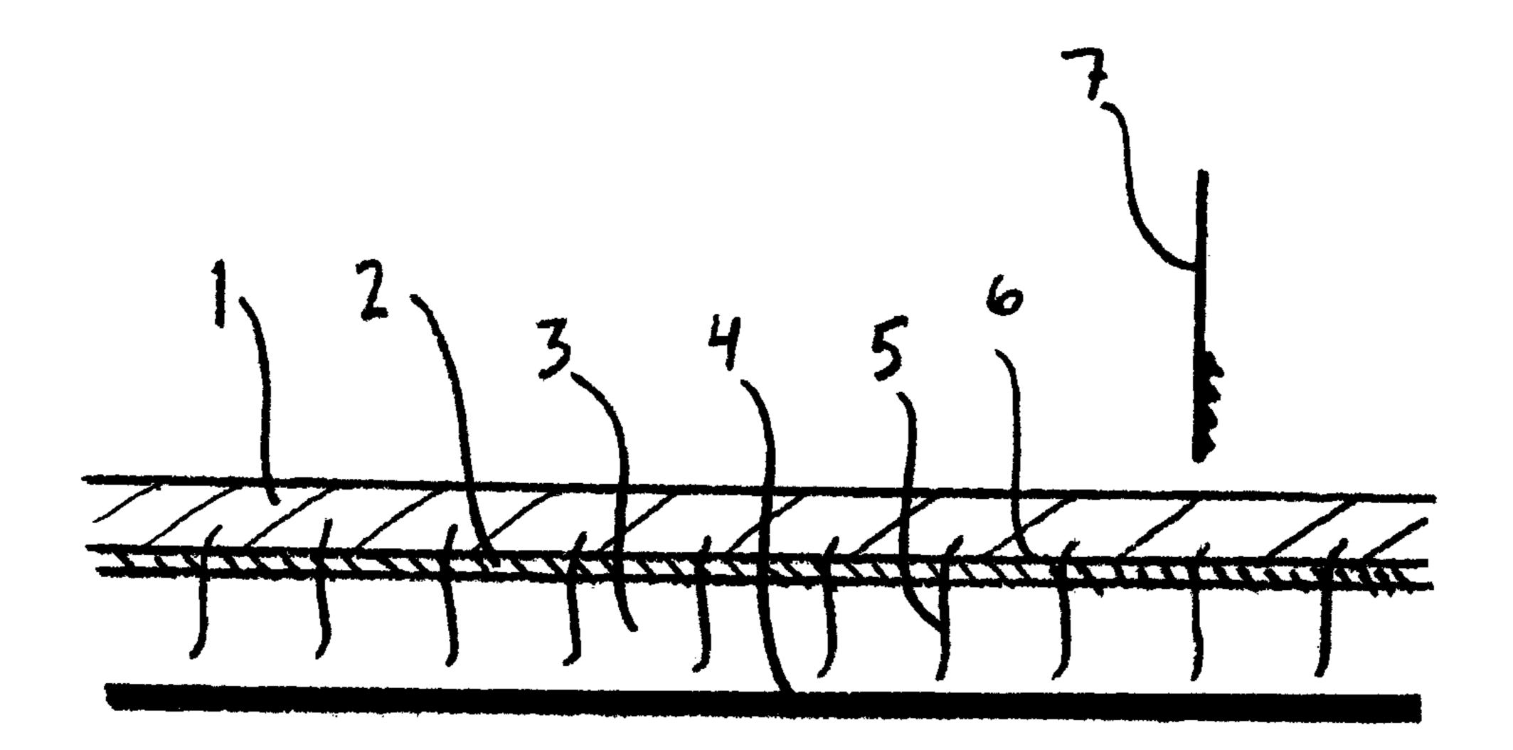
This invention relates to a cured-in-place pipe liner and a method for its production. A cured-in-place pipe liner (CIPP)
