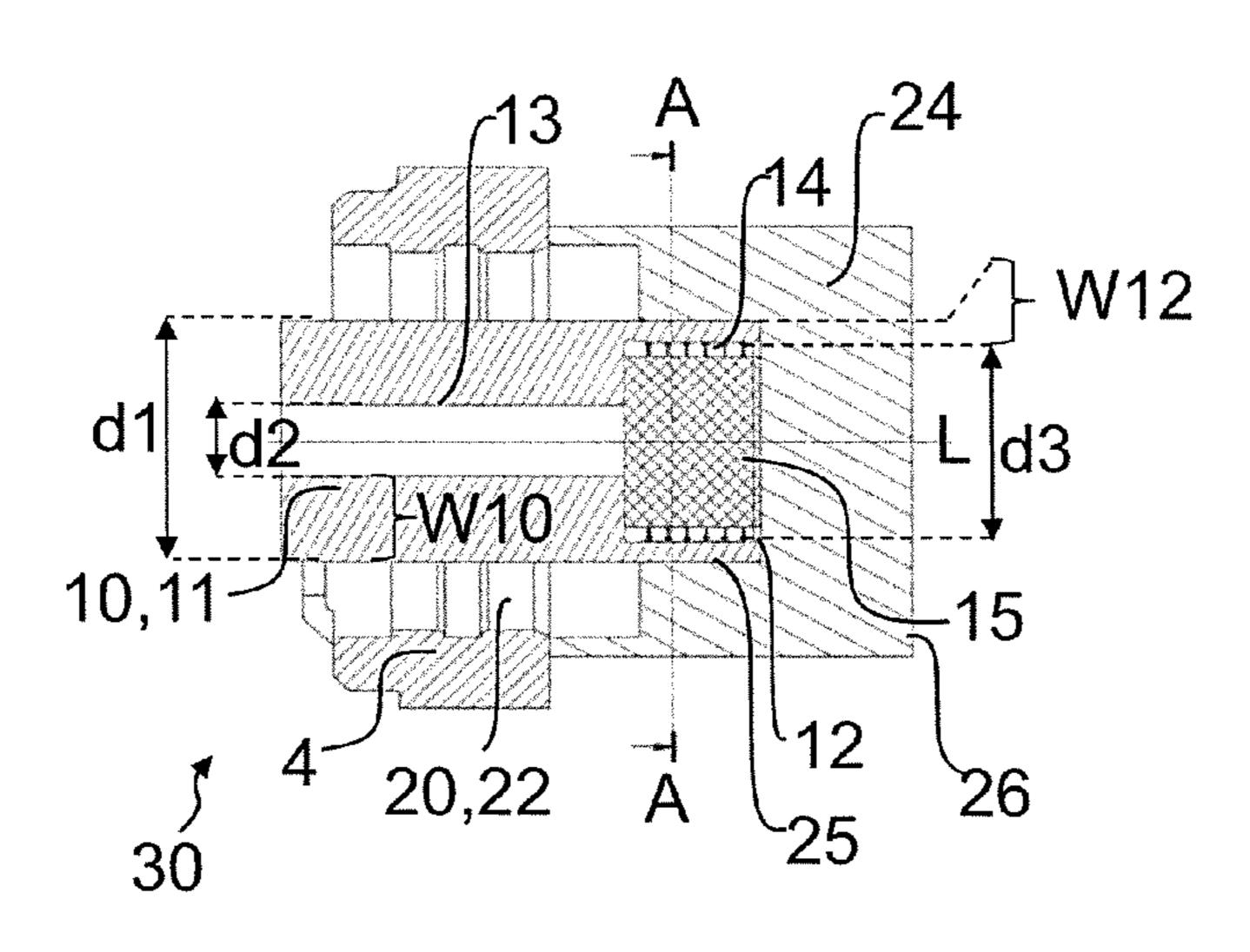
rotary pistons each include a seating for the drive shafts. The respective drive shaft is arranged and fixed with an end region in the seating of the respective rotary piston. A diameter of the drive shafts in the end region can be widened elastically. In an operational state, in which the rotary pistons are arranged on the respective drive shafts, a frictional connection is formed between the respective seating of the rotary piston and the end region of the respective drive shaft.
