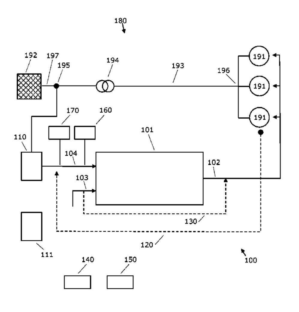
data are used in the power plant controller for determining setpoints for controlling the wind turbine generators' production of active and reactive power. In response to detection of a communication fault a new setpoint is determined independently of new measured grid data by reconfiguring parts of the power plant controller.
