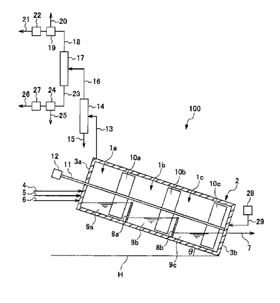
housing chamber. The reaction cells are sequentially connected, and the reaction mixture sequentially moves to each reaction cell.
