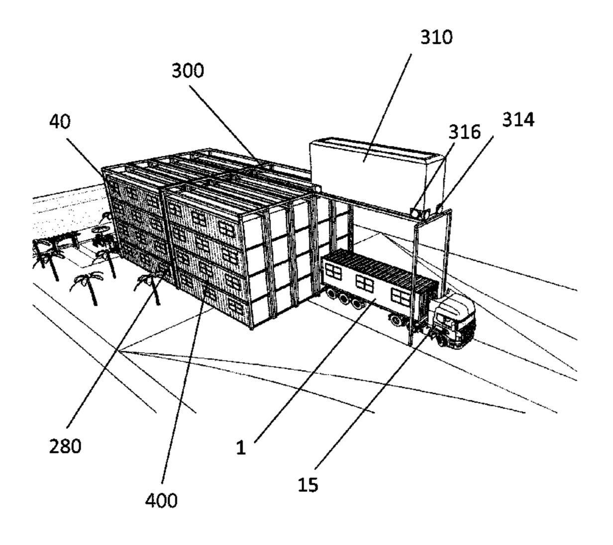
ciated with a number of residential or commercial uses are moved in to and out of the stacks by the robotic handling devices running on the grid. The containers disposed in the stacks are selected by function on demand by a user. In this way the building is reconfigurable to take in to account required uses.
