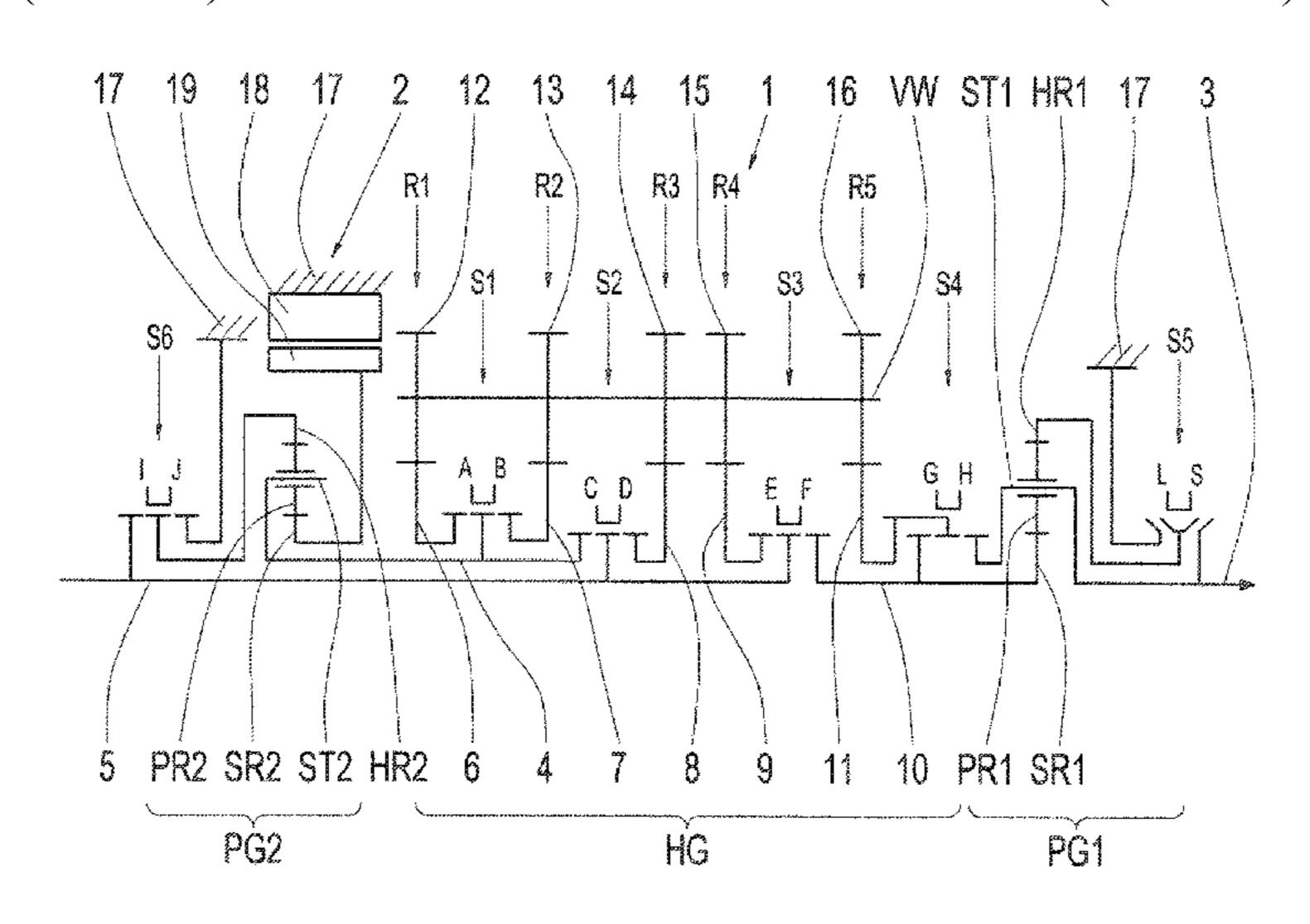
shifting elements (S1-S4). The electric engine (2) is connected to carrier (ST1) of the range group (PG1) and the output shaft (3) so that the electric engine (2) supports tractive force while the range group (PG1) is shifted, and the fifth gear plane (R5) is connected to carrier (ST1) of range group (PG1) and thus can be shifted under load.
