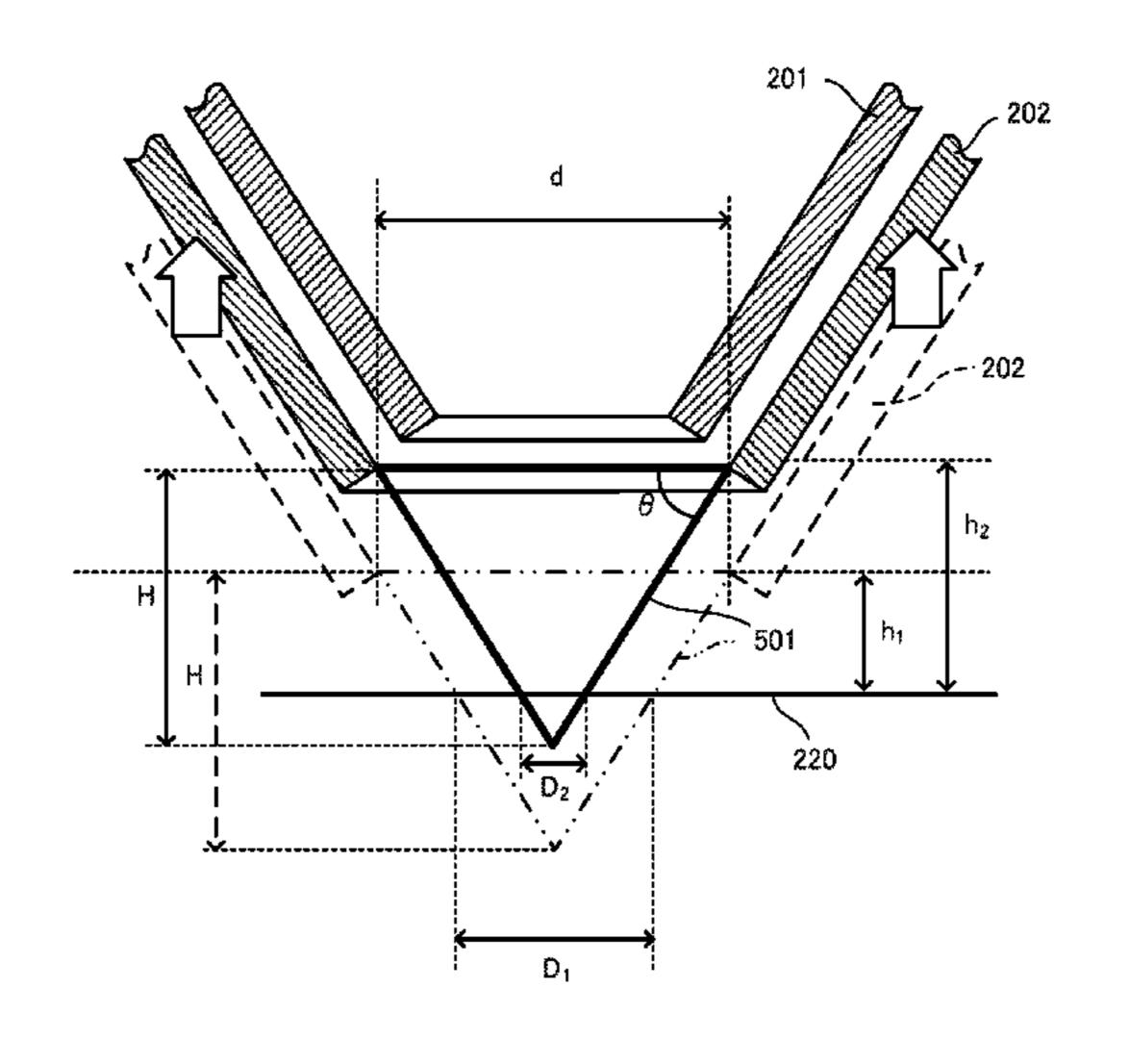
ejection direction of the energy line ejected from the inner housing. The processing nozzle also includes a slide mechanism that changes, along the energy line, the relative position of the outer housing with respect to the inner housing.
