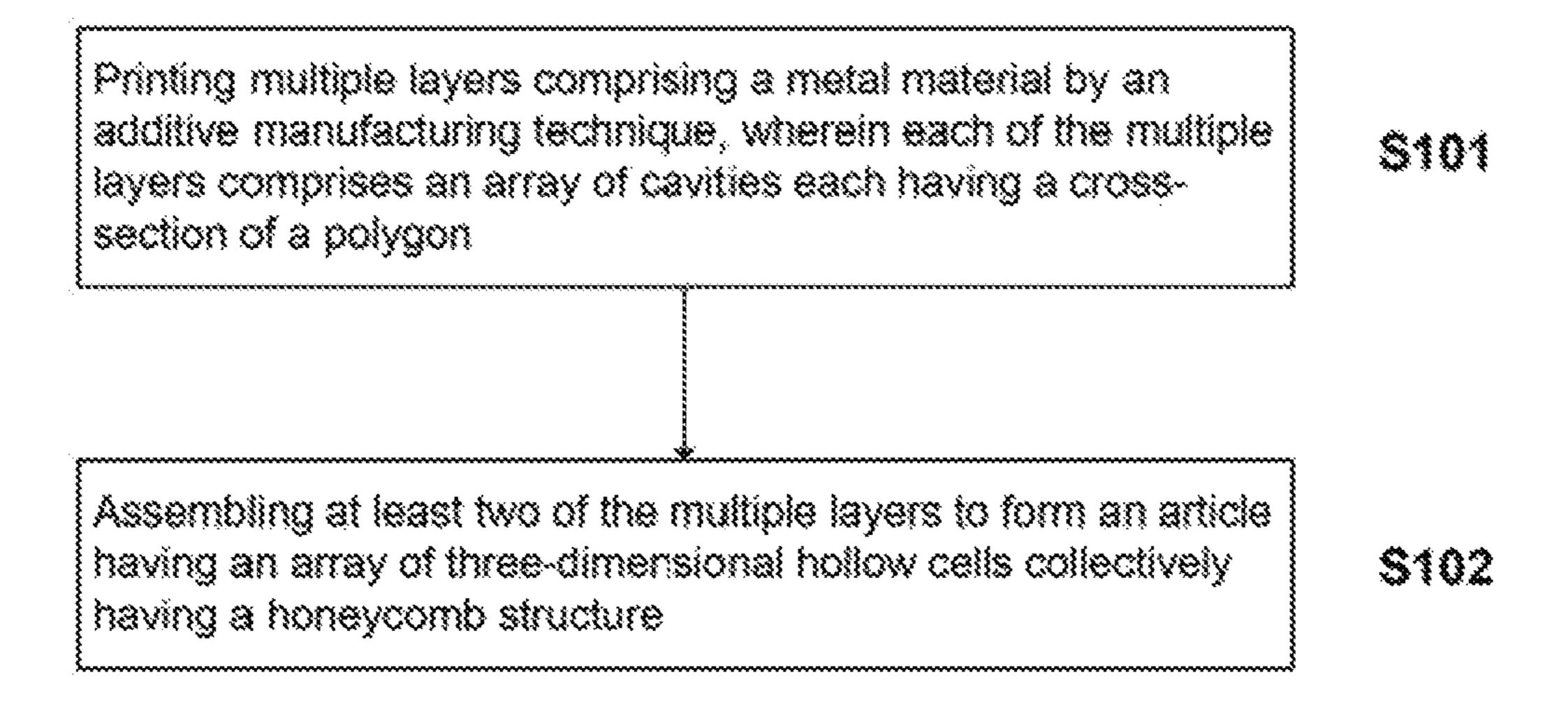
Making a portion of a housing of an electronic device having an electrical circuit, wherein the making comprising:
