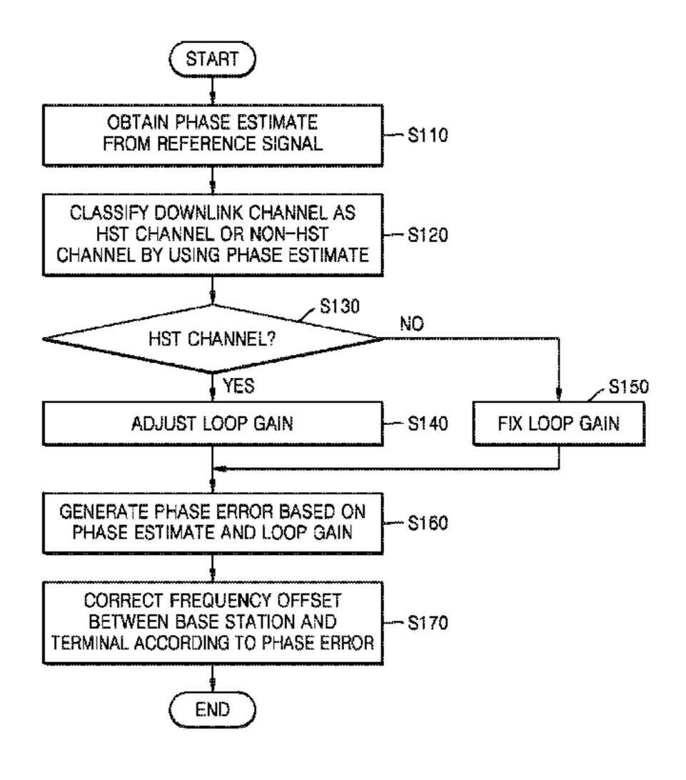
signal received from the base station; classify a downlink channel as a High Speed Train (HST) channel or a non-HST channel based on the phase estimate; adjust a loop gain according to the classified downlink channel; calculate a phase error based on the phase estimate and the loop gain; correct the frequency offset using the phase error; and communicate with the base station after correcting the frequency offset.
