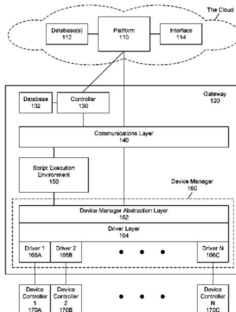
using a communication protocol to read and/or write device properties of the physical device, and a device manager that maps device properties referenced in the virtual-machine programs to device properties used by the driver(s).
