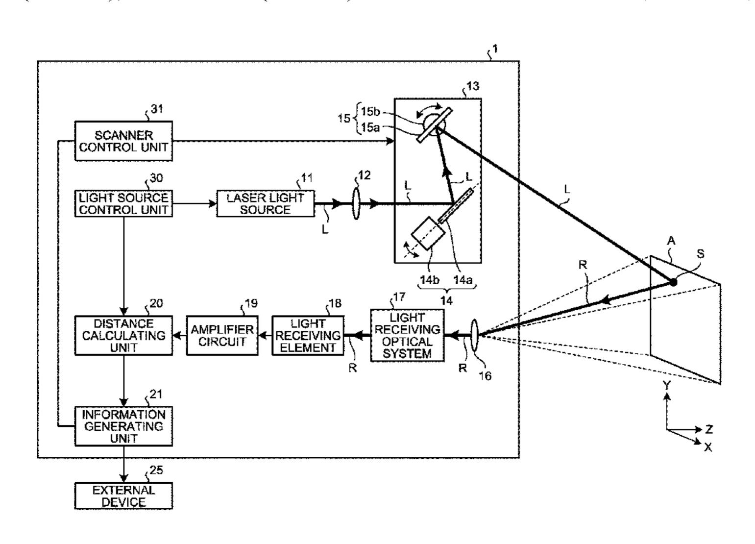
erate, based on a received signal output by the light receiving element, three dimensional information of the area to be measured.
