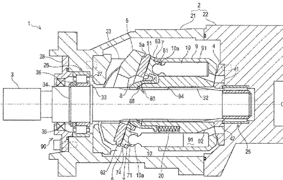
restricts a movement of the rotating shaft relative to the casing toward the first side in the axial direction.
