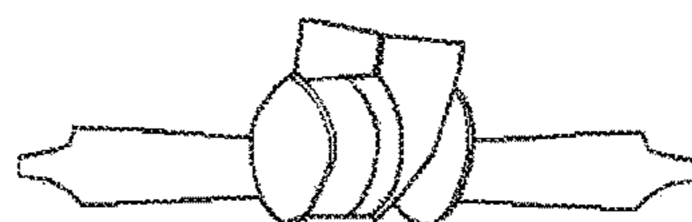
6. WASHER POSITIONED BETWEEN HUB AND TOOTH, DEVICE AT REST
