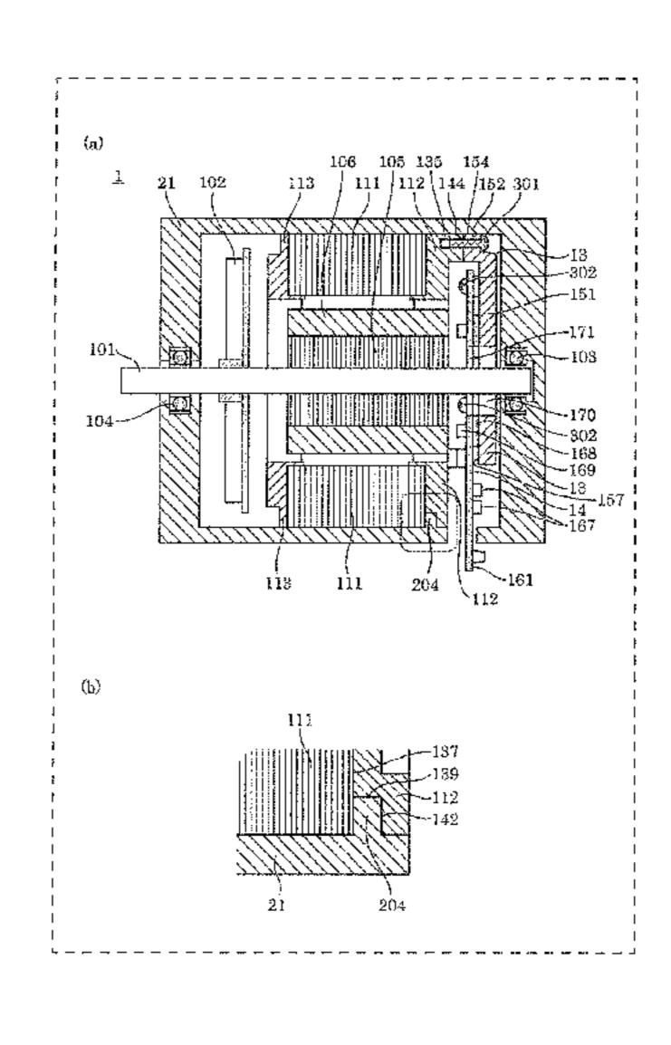
insulator without being in contact with the iron core, and the circuit board is attached to the heat dissipating plate in a state in which the circuit board is in contact with the heat dissipating plate without being in contact with the iron core.
