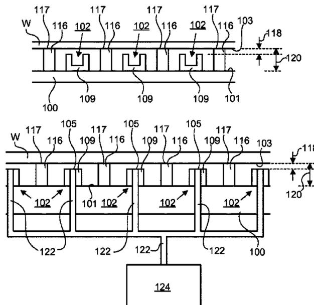
and configured such that a lowering of the substrate into a position on the support table at which the substrate is supported by the support table causes a localized build-up of pressure within the recess. The localized build-up of pressure provides a localized gas cushioning effect during the lowering of the substrate.
