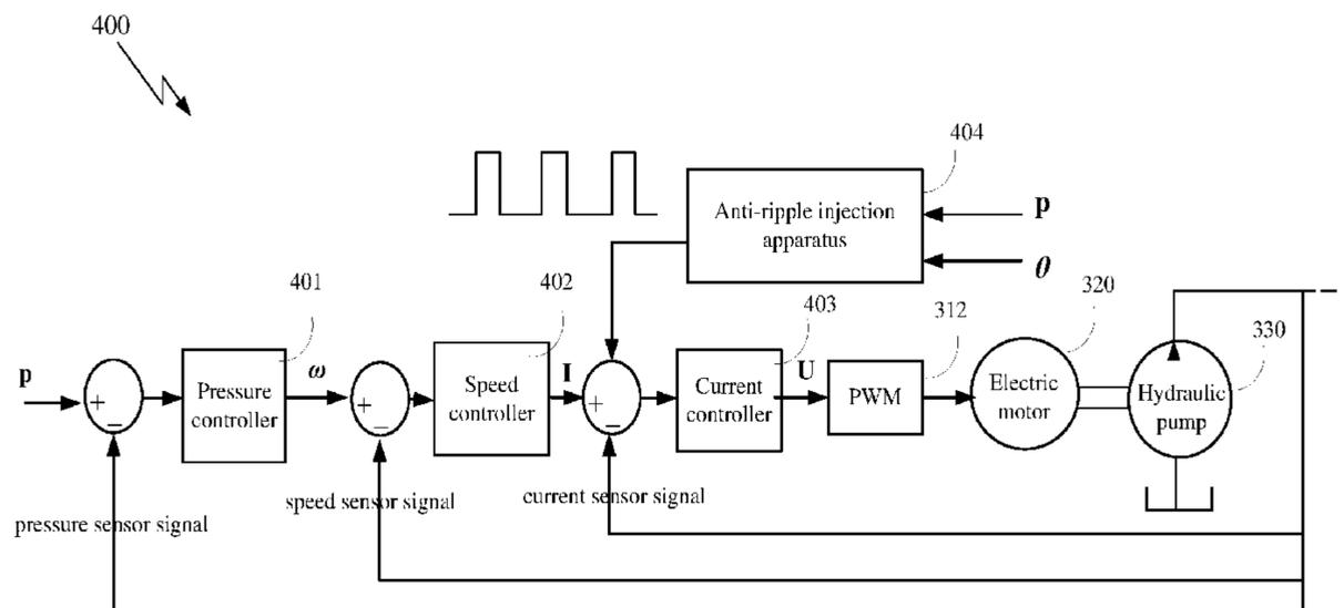
anti-ripple injection apparatus, and a pump system including the control system are also disclosed.
