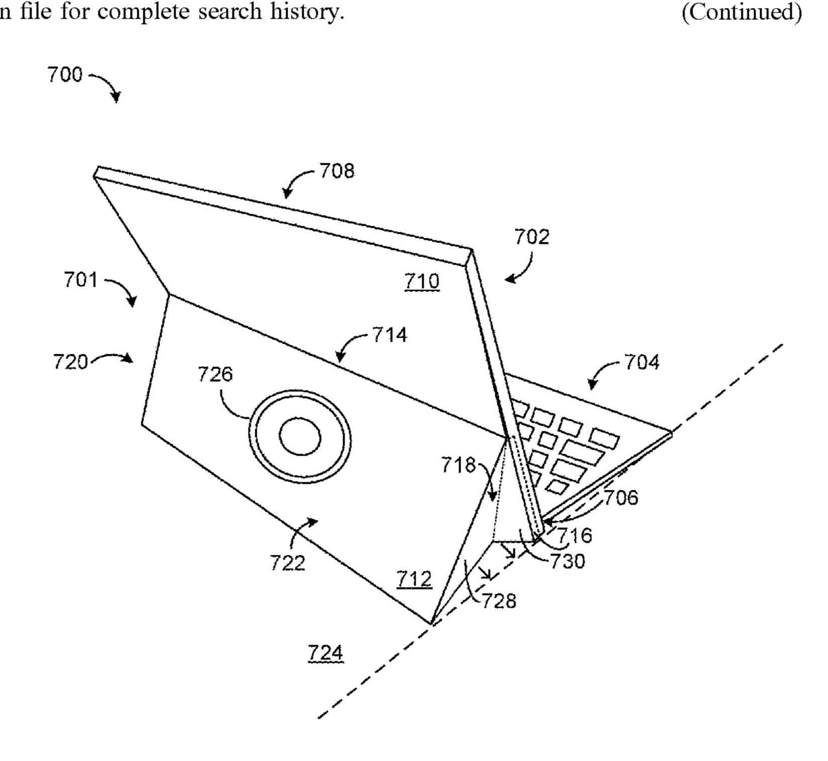
faces an exterior of the resonance box. In this way, the electronic device gains the benefit of amplifying audio via the resonance box without adding significantly to the device volume or requiring an auxiliary speaker system.
