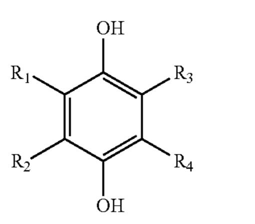
where in Formulae I,  $R_1$ - $R_4$  may be substituted or unsubstituted alkyl or aryl groups, or heteroatomic groups containing hetero atoms of Groups V-VII of the periodic table, and substituents  $R_1$  and  $R_2$  (taken together), and/or  $R_3$  and  $R_4$ , may form a ring.
