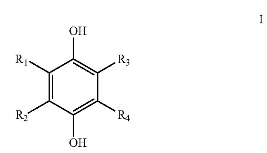
wherein, in Formulae I,  $R_1$ - $R_4$  may be substituted or unsubstituted alkyl or aryl groups, or heteroatomic groups containing hetero atoms of Groups V-VII of the periodic table, and substituents  $R_1$  and  $R_2$  (taken together), and/or  $R_3$  and  $R_4$ , may form a ring.
