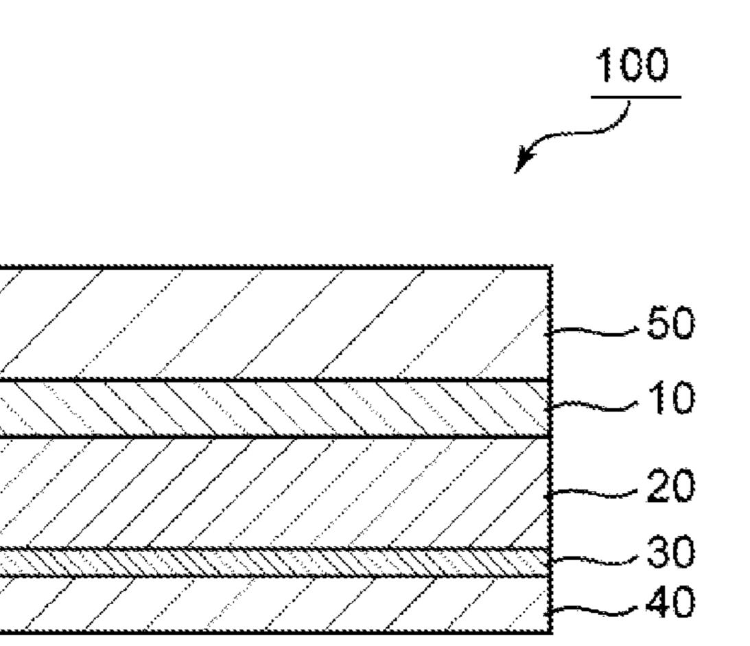
a barrier function. An angle formed between an absorption axis of the polarizer and a slow axis of the retardation layer is from 35° to 55°.
