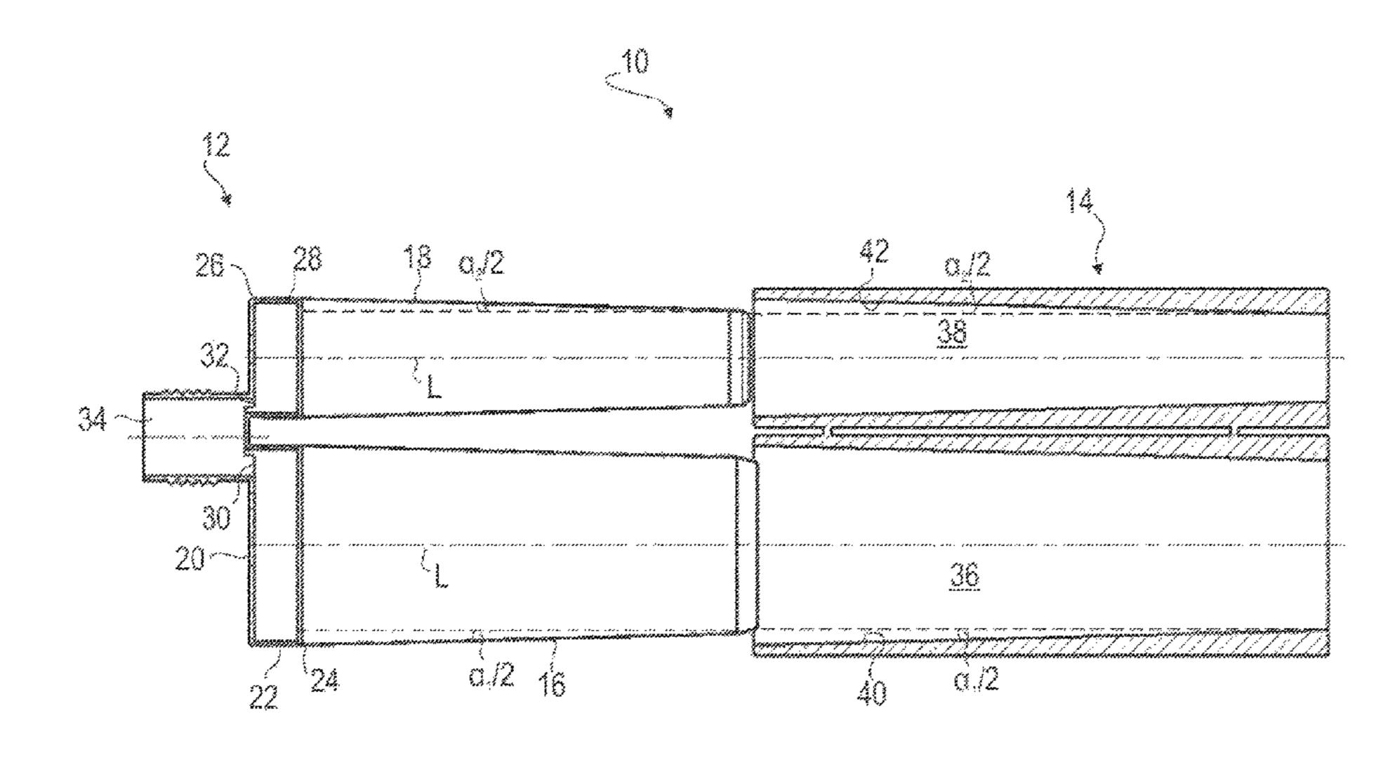
form of a truncated cone, the diameter of which narrows in the direction of a longitudinal axis, starting from the respective fastening portion.
