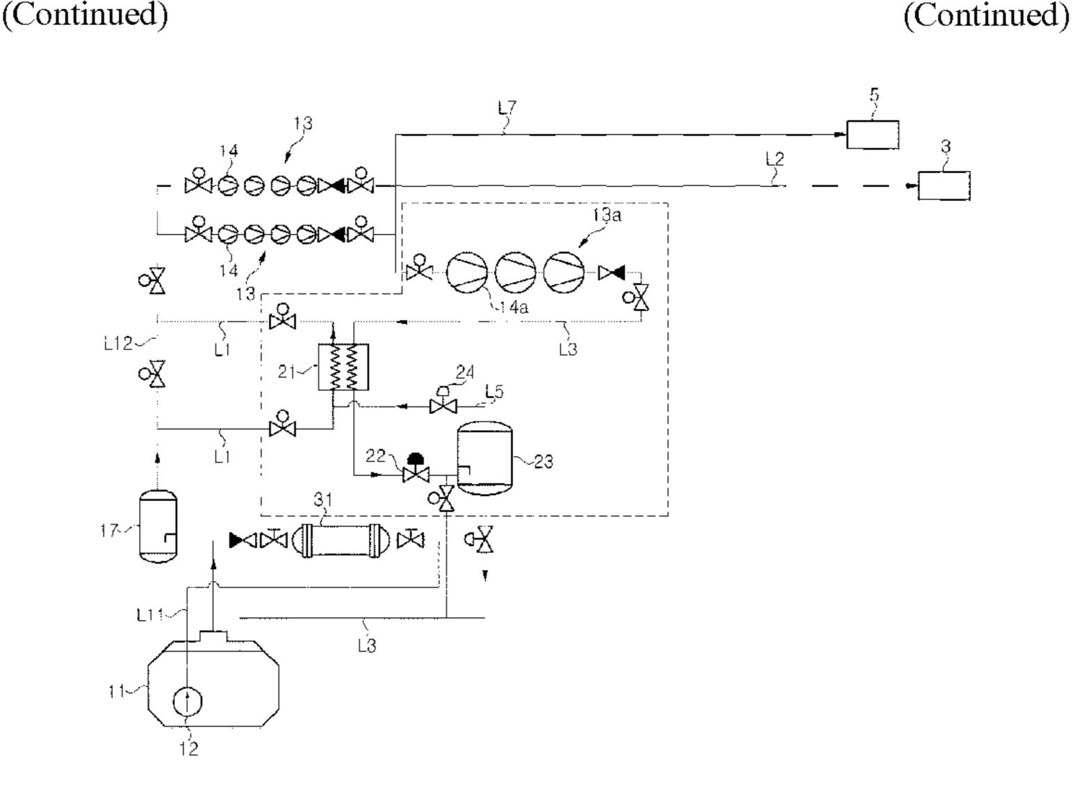
gas engine receiving at least a part of the BOG compressed by the compressor, as fuel; a heat exchanger exchanging heat between the remaining part of the BOG, which is not supplied to the medium pressure gas engine as fuel, and the BOG, which is discharged from the storage tank and is not compressed; and an expander decompressing the remaining part of the BOG cooled by the heat exchanger.
