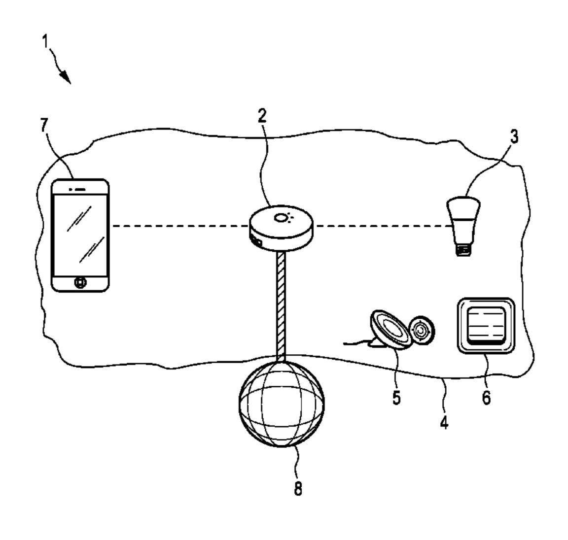
in the wireless network in response to the detection of the device, and retrieves the digital asset from the upgrade server of the device. This leads to an improved way of integrating the device into the connected device system.
