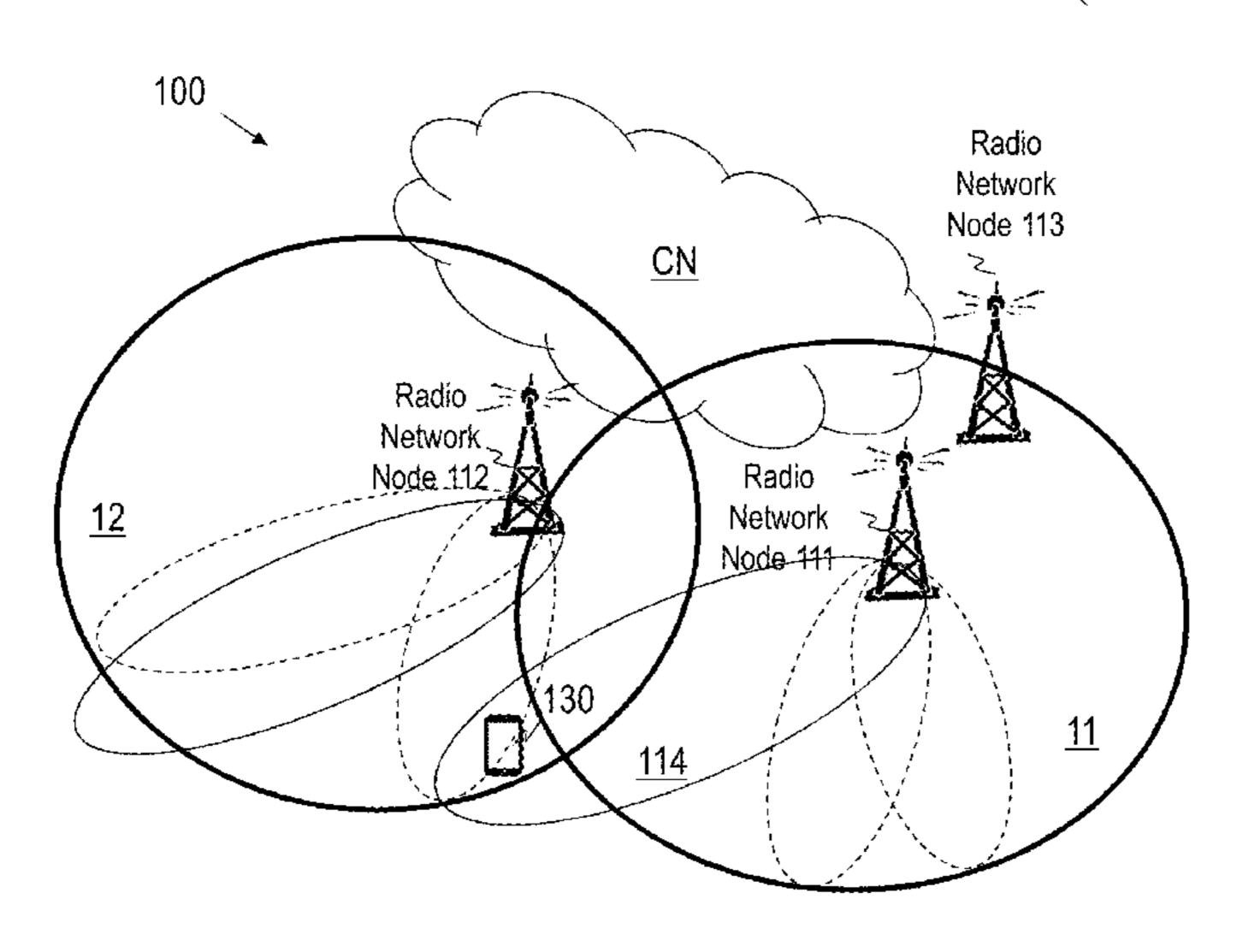
nodes and stores information on active mode beam to idle mode cell relations, wherein the active mode beam is the beam serving the user equipment (130) when a new synchronization signal is detected, and the idle mode cell is the cell with the synchronization signal broadcast area provided by the network node transmitting the detected synchronization signal.
