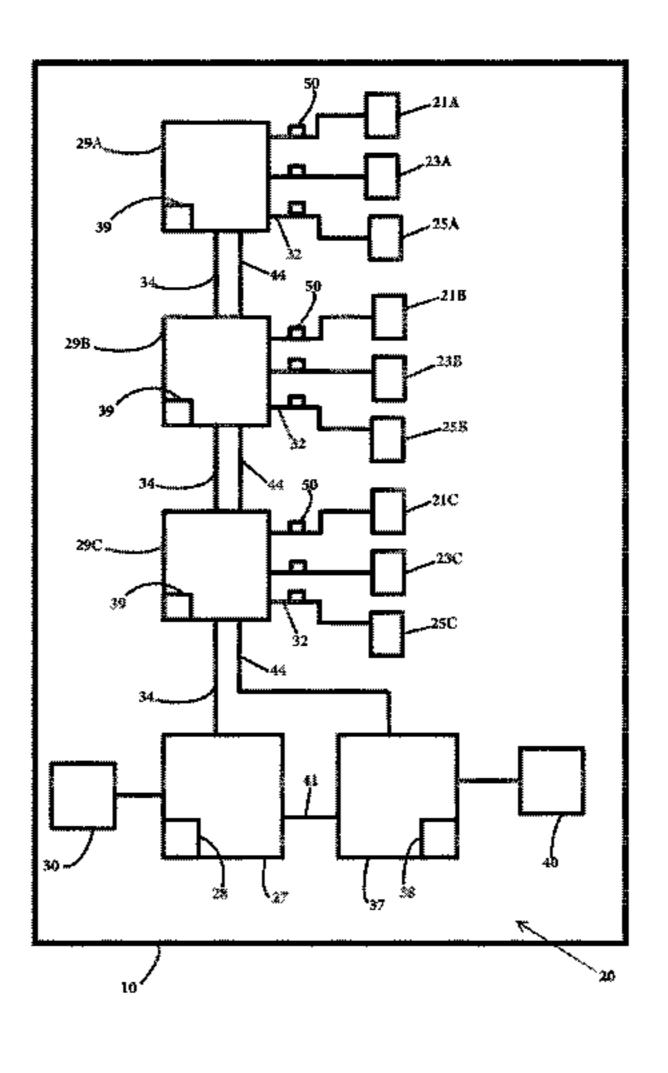
detected that the standby control unit is also not operational, the plugin modules switch to an autonomous mode such that operating instructions for the climate output devices and air inlets are determined by the plugin modules.
