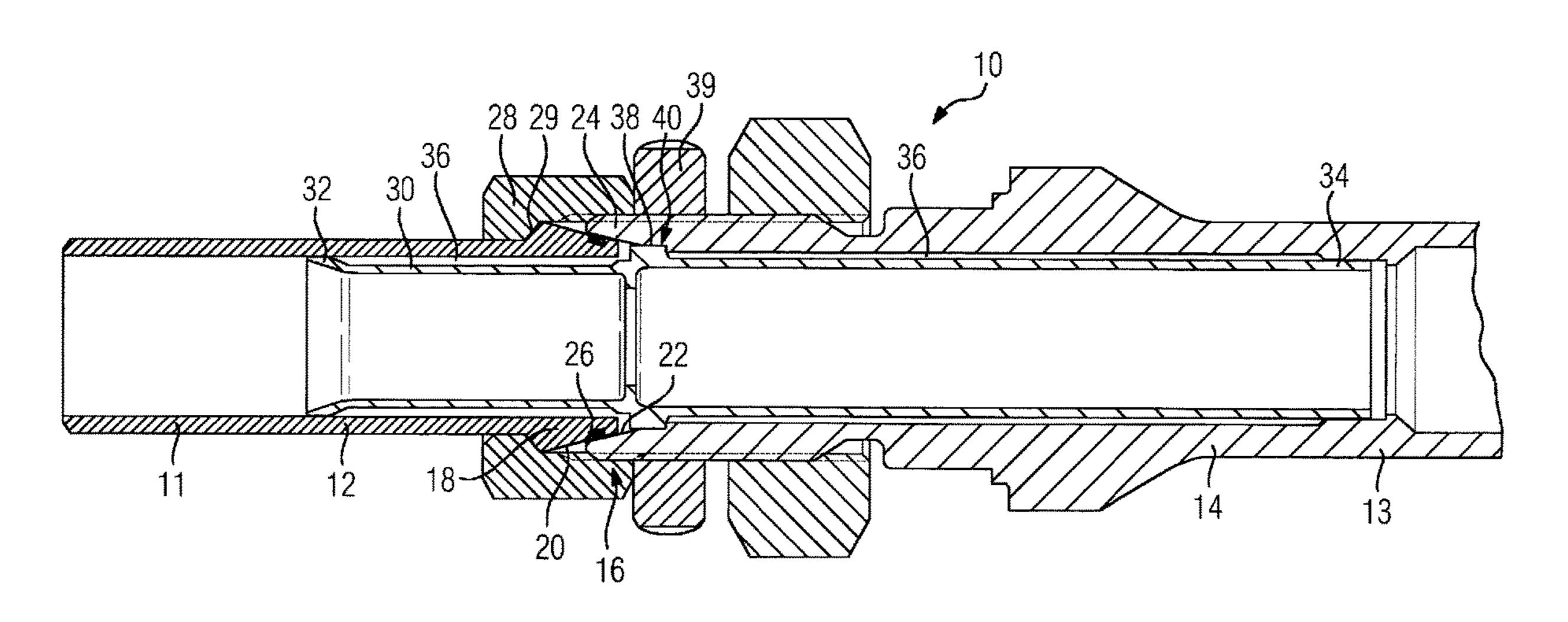
annular groove is provided in one of the sealing surfaces. In order to enable the pipe connection also to conduct a fluid having cycling or varying temperature, the inner of the two connection parts has thermal insulation on the inside of the pipe at least in the axial segment of the sealing surface of the connection part, wherein the thermal insulation tube has a cam or a collar on the outer surface, which engages in a recess, which is axially bounded by the two connection parts.
