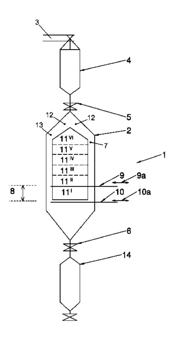
removed by force of gravity. Using biomass feedstock that has been compressed in a reciprocating piston press to bulk density of at least 500 kg/m3, which can be fed dry into the reactor using simple, inexpensive sluice systems and then wetted inside the reactor, this system provides comparable biomass throughput at a fraction of the cost of traditional commercial hydrothermal pretreatment systems used in "second generation" biorefining.
