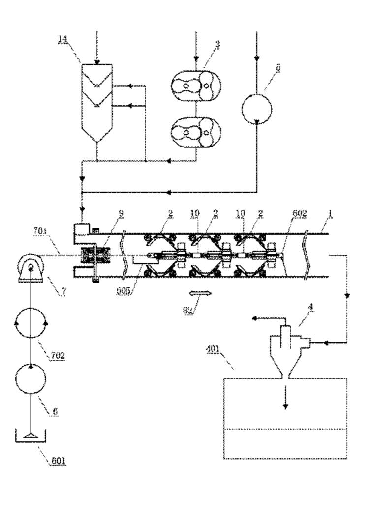
rotation nozzle of a turbine crawler which moves inside the pipe, thereby polishing the inner surface of the pipe, and following the polishing work, the turbine crawler can clean, dry and coat the inner surface of the pipe.
