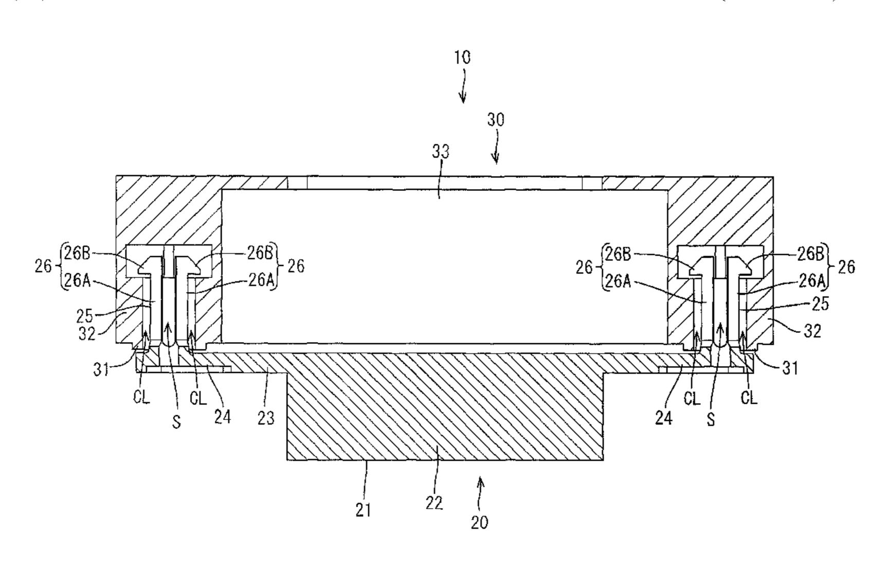
hold the mounting pin in a state in which it is inserted into the corresponding mounting recess. The mounting pin is capable of relative movement inside the mounting recess in directions that intersect a direction in which the mounting pin is mounted into the mounting recess, and the mounting pin is provided on one or two of the outer peripheral sides of the housing.
