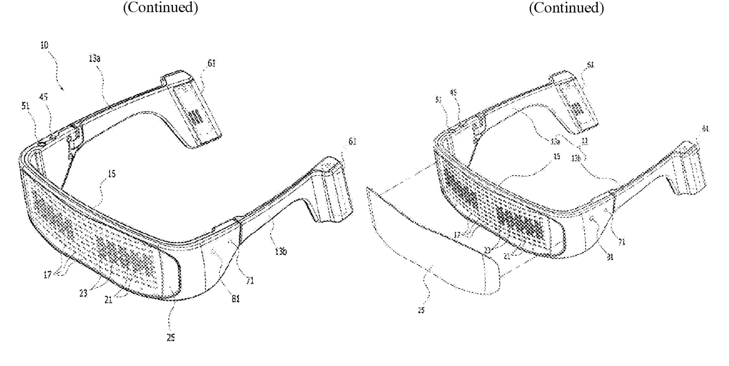
openings are arranged in a plurality of lines, each line of openings is parallel along a lengthwise direction of the front frame, lines of openings are positioned at each of a left-center portion and a right-center portion of the front frame.
